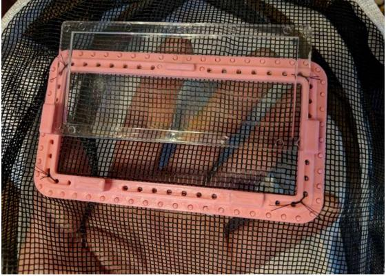
Step 7. Insert lens under the tabs on left and right sides. Slide all the way down until it snaps into place.
